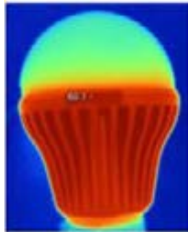
Figure 13: Steady-state infrared thermal image of MX-6 A19 lamp
