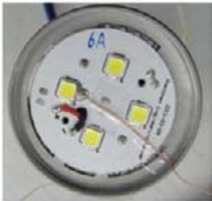
Figure 11: Thermocouple attached to MX-6 LED
