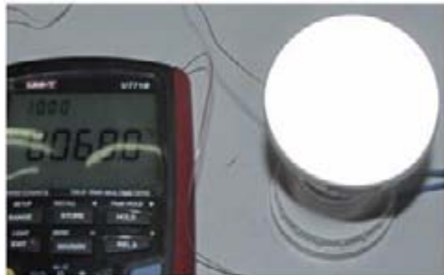
Figure 12: MX-6 A19 solder-point temperature measurement
