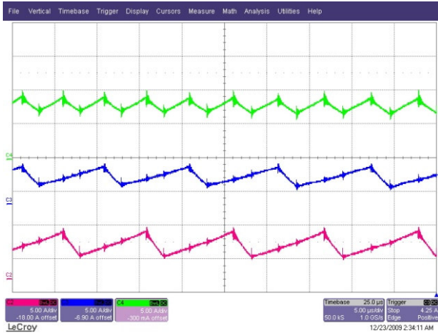
Figure 3: Input and Inductor Current Ripple at V_{in}=85V RMS and P_{out}=650W
