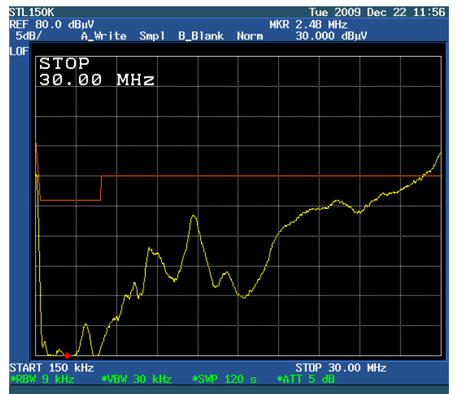
Figure 11: Frequency sweep from 150kHz to 30MHz Vin=208V RMS and Pout=650W
