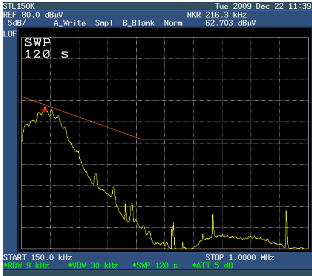
Figure 8: Frequency sweep from 150kHz to 1MHz Vin=208V RMS and Pout=650W
